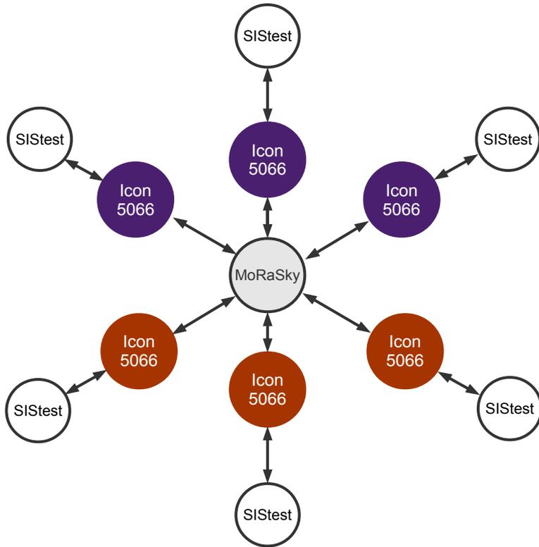
MoRaSky simulates HF Modems, Radios and the Ionosphere.
